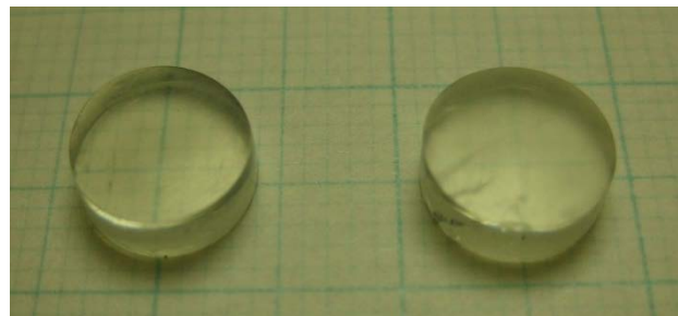
Fig. 2: Photograph of 40 wt% (left) and 60 wt% (right) \text{HfO}_2 nanoparticle-loaded plastic scintillators, approximately 8 mm in diameter and 3 mm in thickness.
